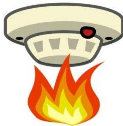
Smoke alarms are devices that are able to detect smoke or fire then sound an audible alarm. They are very useful in detecting a fire in its early stages, allowing you adequate warning to evacuate before inhaling any harmful gases. For the best protection, install both ionization and photoelectric smoke alarms (some models provide dual coverage). **Smoke alarms should be installed on every level of your home or apartment building.**
